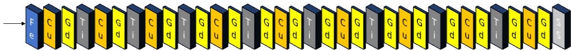
Figure 3.1. Visualization of foils stack implemented in this work. All Gd foils were encapsulated in Kapton tape.
